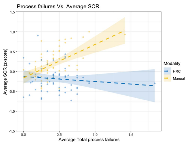
Fig. 11 Scatter plot between total process failures and average SCR comparing Manual and HRC modalities. Dotted lines, with and confidence bands, represent the relationship between the two variables
